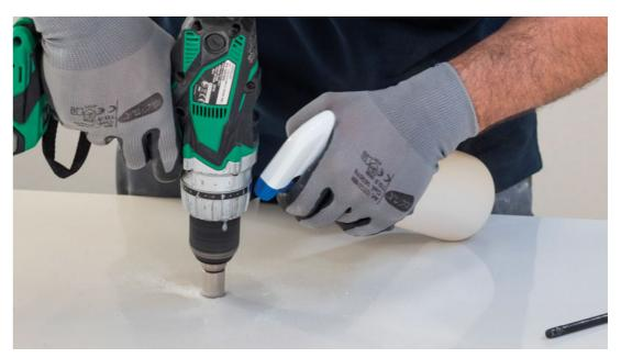
3. Keep the drill/screwdriver at an angle of 90° and, applying gentle, constant pressure, make circular movements at an angle of about 5°-10°.
