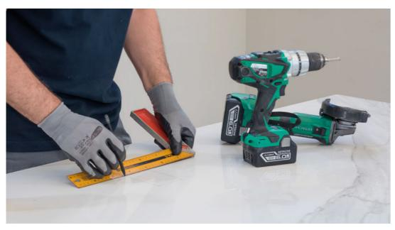
1. Marking: mark the part to be cut off on the slab.
