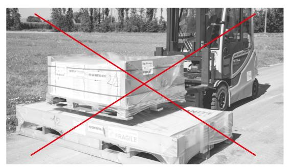
To prevent damage to slabs, do not stack items of different sizes on top of the crates.
