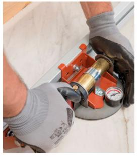
2. Before handling, ensure that the suction cups are adhering firmly to the slab.
