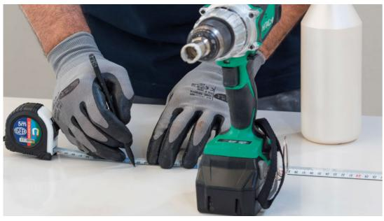
1. Place the Mega slab on a hard, firm, non-slippery surface such as wood or concrete. Wet the area where the hole is to be drilled with water.
