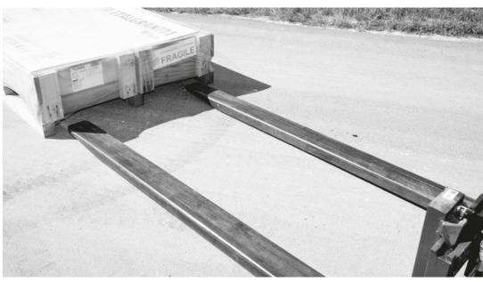
**B**. For correct handling of the pallet on the short side (e.g. when unloading containers), forks at least 2.5 metres long should be used to ensure that the material is held perfectly and safely.
