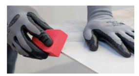
**Diamond pads** for finishing edges After cutting.
