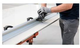
**Cutting guide with scorer** for linear and diagonal cuts up to 320 cm.
