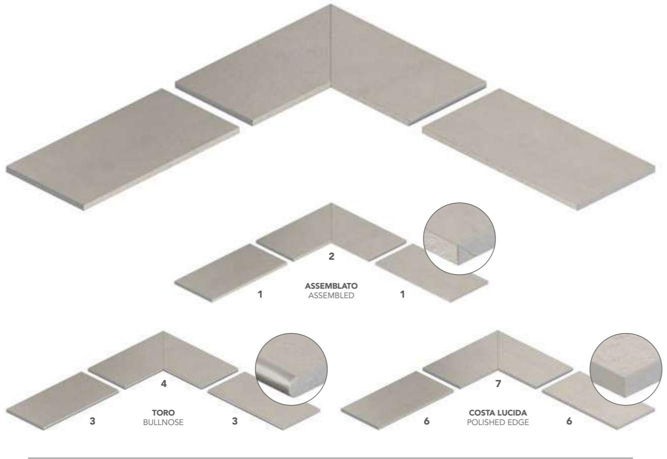
**POSA CON ANGOLO CURVILINEO / ROUND CORNER INSTALLATION**
