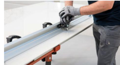
**Cutting guide with scorer** for linear and diagonal cuts up to 320 cm.
