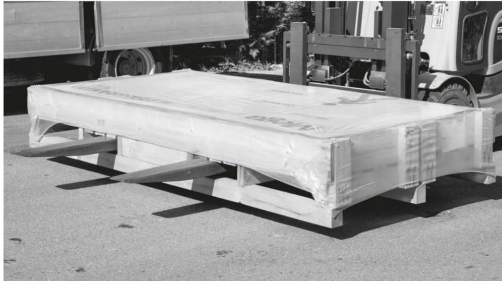
A. For correct handling of the pallet on the long side, the forks must be widened to their maximum setting and placed in the centre of the pallet; ensure contact through the entire depth before lifting.
