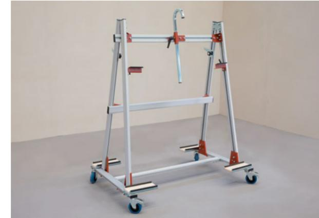
Handling trolleys designed to allow application of adhesive to the back of the slab.
