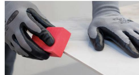
**Diamond pads** for finishing edges After cutting.
