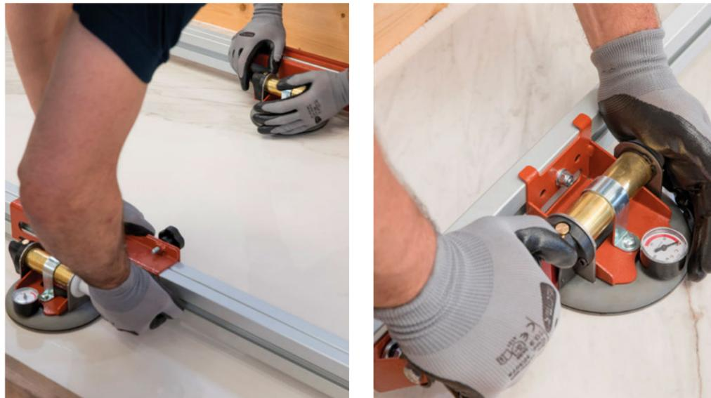
2. Before handling, ensure that the suction cups are adhering firmly to the slab.
